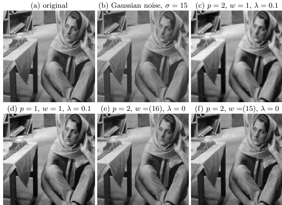
Fig. 1. Application to image denoising. Regularizations performed with t = 5 . (c) Unweighted L_2 regularization (13) on an 8-adjacency graph. (d) Unweighted TV regularization (13) on an 8-adjacency graph ( p = 1 ). (e) Regularization (13) with p = 2 and weight function (16) and scalar feature F_f = f on an 8-adjacency graph. (f) Regularization (13) with weight function (15) and feature vector F_f(v) = [f_u : u \in B_{v,7}]^T on an \epsilon -neighborhood graph with \epsilon = 4 .
